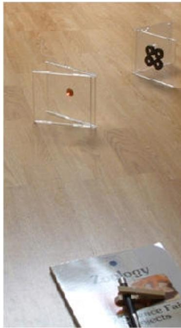
*A laser pointer beam is aimed at the mirror of the magnetometer. The case with four magnets at upper right nulls the Earth’s magnetic field, so the device measures outside influences.*
