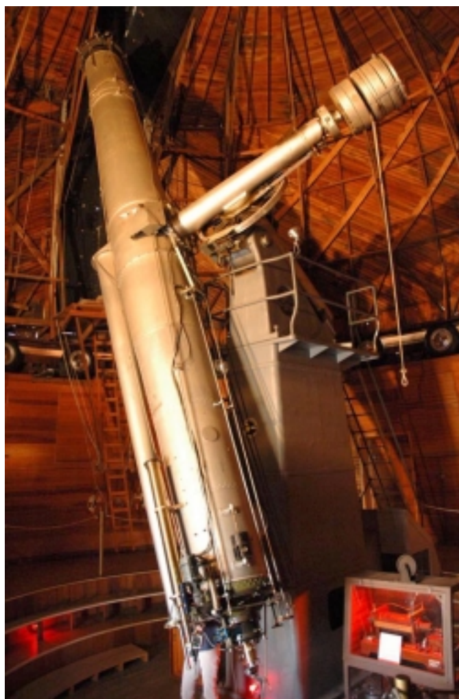
The 24-inch Alvan Clark Refracting Telescope, inside the dome of the Lowell Observatory. The dome, constructed of pine and fir, rotates on 1952 Ford pickup tires! Photo by Burley Packwood.
