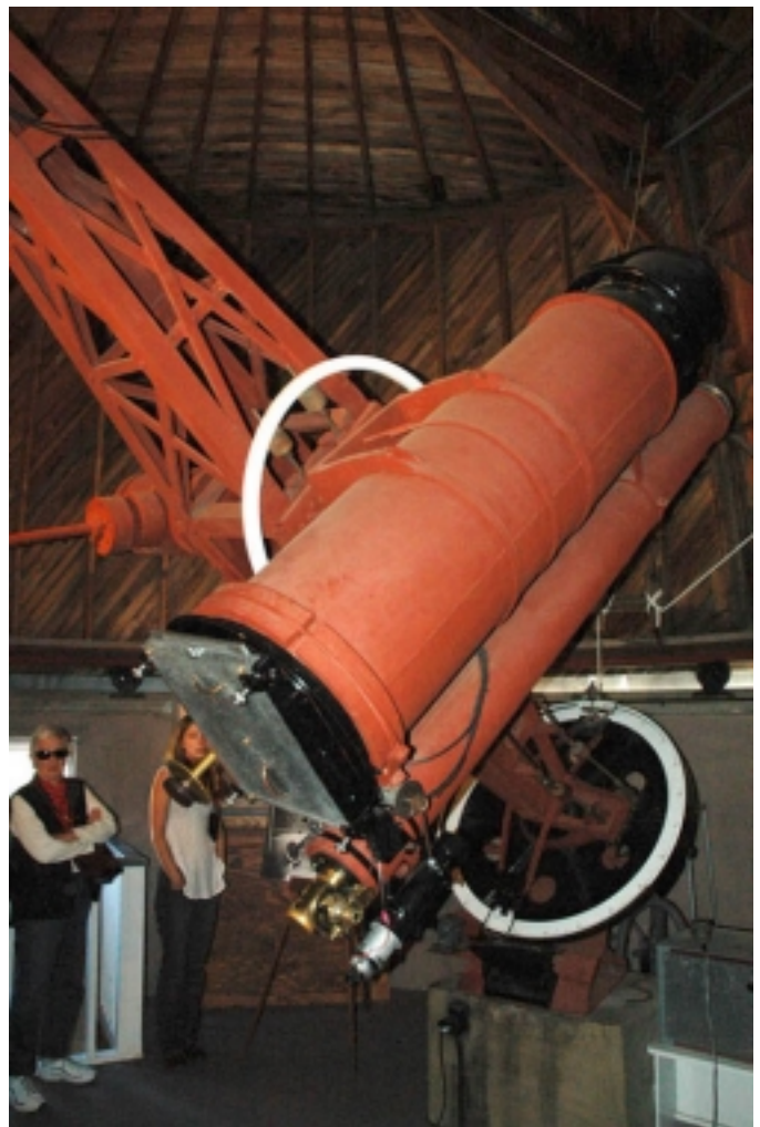
This 13-inch Astrograph telescope was used by Clyde Tombaugh to discover Pluto. Photo by Burley Packwood.
